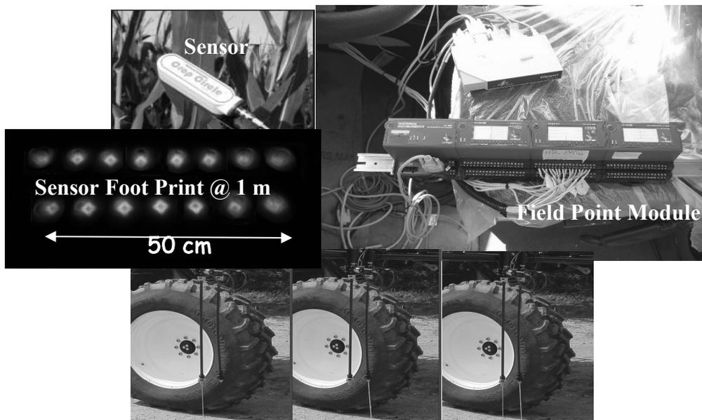
**Fig. 2.** Key system hardware components include a Holland Scientific Active sensor, Field Point Control Module that is interfaced to the sensors and PC running software that is controlling electronic valves delivering varying amounts of liquid N fertilizer.
